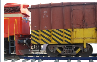
In motion Rail Weigh Bridge
